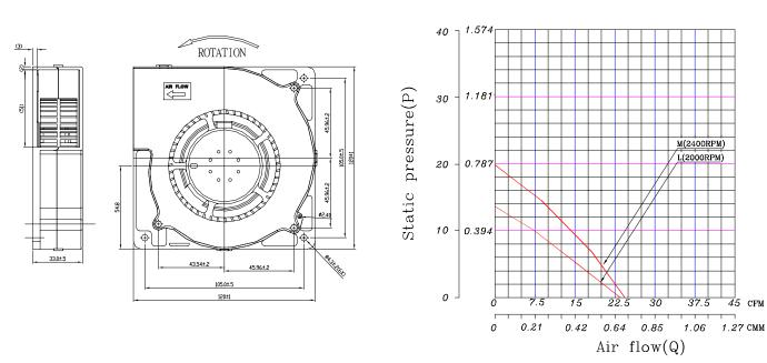
Air exhaust radial, through housing port. Rotational direction CW looking at rotor.
